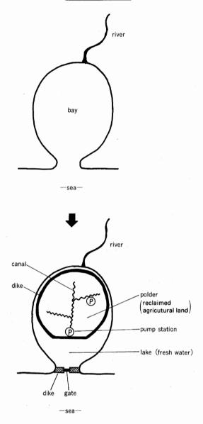
Figure 6 Sea bottom reclamation double dike system.
